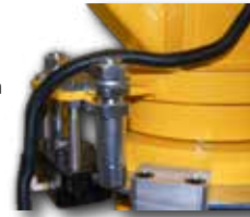
Parking brake and main rotation stops
