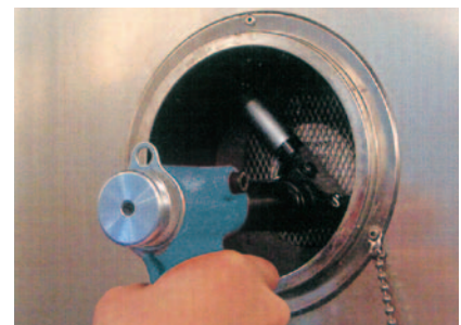
90 Angle nose of AR2000A-90 allows to riveting inside of the cylinder, shown as picture
